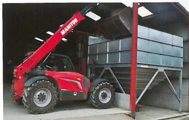
*Having the dryer and bin on a lower level gives the forklift driver a better view of the bin when he's loading it.*
