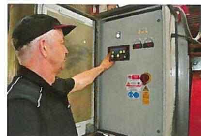
*The dryer is programmed using a touchscreen which is easy to understand and use – just like a big mobile phone.*
