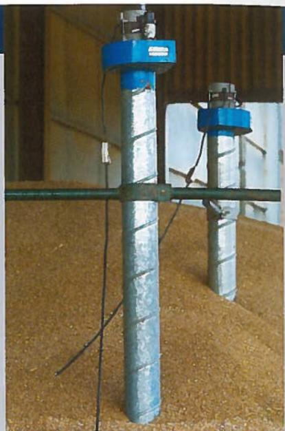
While AHDB recommends an airflow of 6 cubic feet per minute per stored tonne of crop, many farms ventilate as low as 1 cfm per tonne, or not at all.
