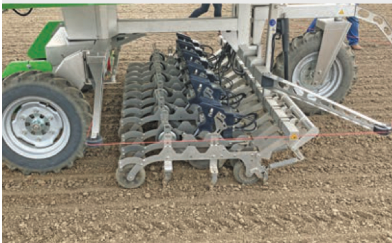
The machine uses a combination of weeding wires and blades to remove weeds between and within rows, based on records of each seed's sown location.
