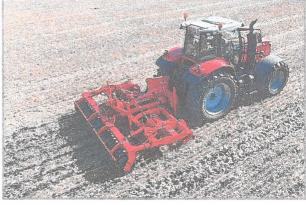
MODERN SUB-SOILERS have very low surface disturbance and can be used to alleviate compaction without disturbing the soil profile. With the HE-VA Stealth, a disc makes a cut and a leg passes through - the soil profile is not inverted
