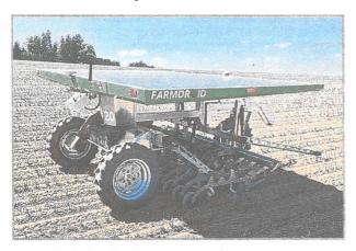
LOW DISTURBANCE tillage, labour-saving robotics and energy-saving electronics, are becoming more commonplace -FarmDroid uses ultra-accurate GPS to record exactly where it places each seed. On each subsequent weeding pass, it has no need to identify what's a weed and what's not - it simply knows where the crop plants should be and works around them
