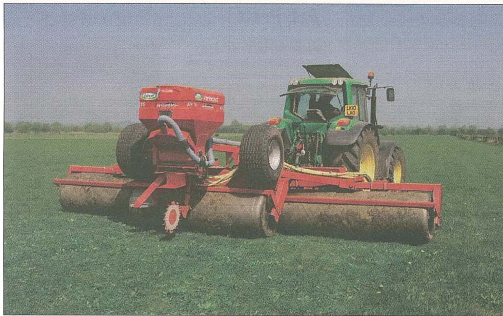
The He-Va 6m roll with harrow and seeder played a crucial role in improving the grassland.
