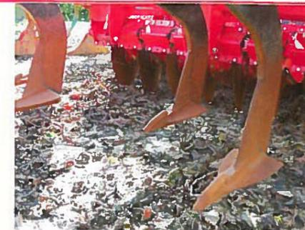
Low disturbance legs to loosen compaction with minimal disturbance were high on Richard Scott’s want list.
