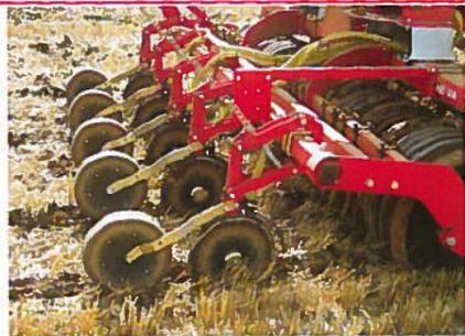
Shown here on a mounted machine, Accu-Disc units combine offset double-disc units and following press wheels.
