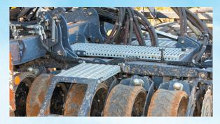
Above: The drill's depth is adjusted using a turnbuckle system fitted above the front press wheels
