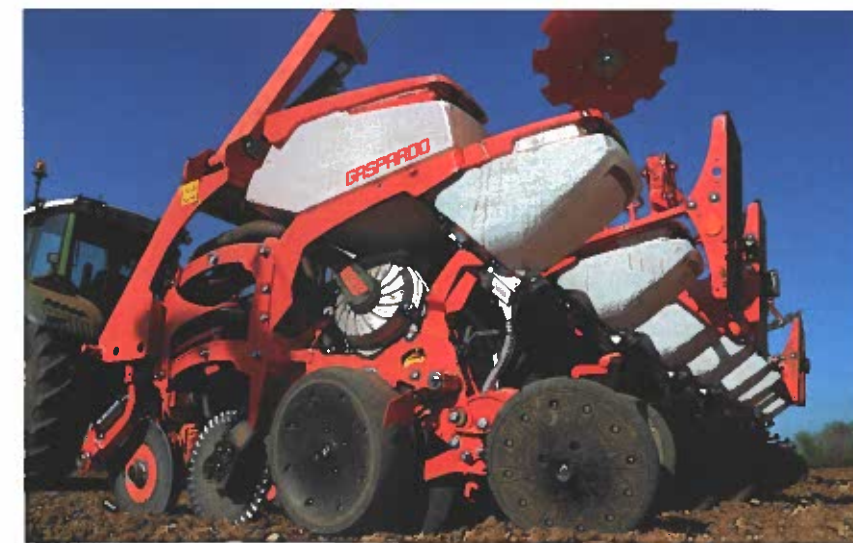
The singulation system uses a fan-driven vacuum to hold the seeds onto the plastic disc before they are gravity fed into the chute. Once here, a pneumatic system pushes them to the seeding disc. It's a fast acting system to deal with high forward speeds.
