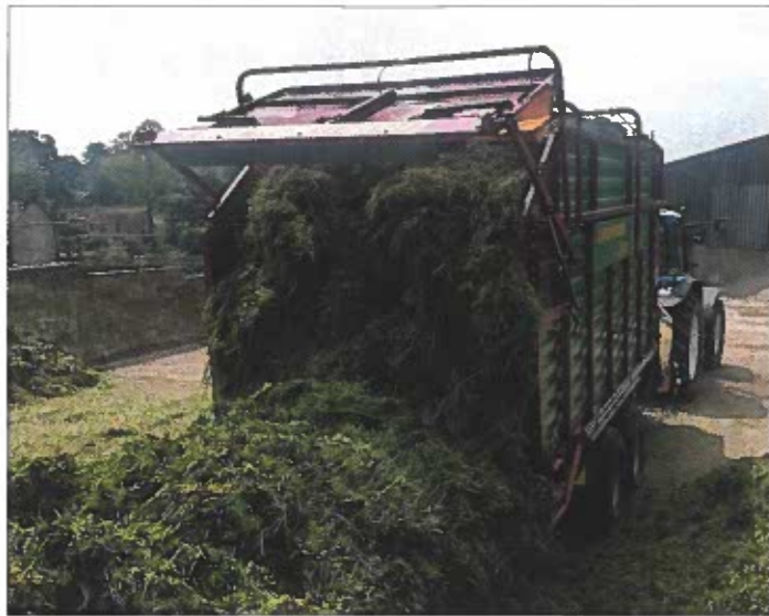
The forage wagon gives a more consistent and longer chop than the silage forager system it has replaced.
