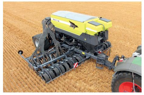
Around this time Sulky moved from its trademark turbine metering units to peg-wheels better able to cope with larger seeds such as beans and peas. These could handle rates as low as 3kg/ha for OSR right up to 300kg for late-drilled winter cereals.
