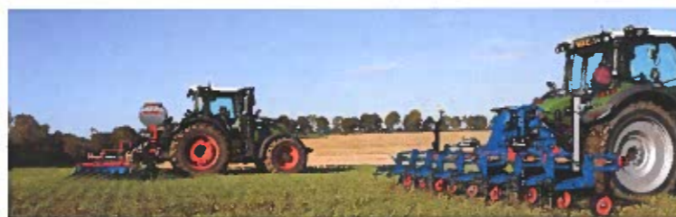
Both of these are mechanical weeding tools, but they do a different job. In the foreground is the hoe, which is designed to work between the crop rows so it needs to be the same width as the drill. The other unit is classed as a comb harrow, with its lighter tines plucking out the younger weed plants, not the crop.
