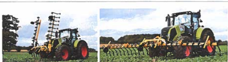
At LAMMA, Claydon will have the 20-tine, 6.0m version of its TerraBlade mechanical weeder. This is an additional heavy-duty model of which there is also an 8.15m, 26-tine version. These join the standard 3.0, 4.0, 4.8m and 6.0m models. All are front-mounted to keep the unit simple and low-cost.
