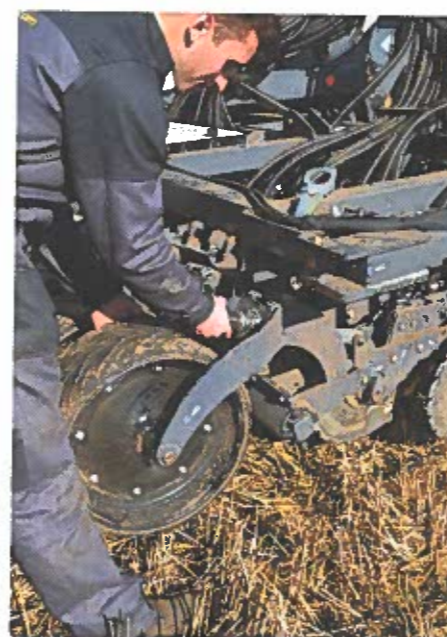
Disc depth adjustment is done by slackening off a nut on the front of each coulter carriage and adding or removing collars.
