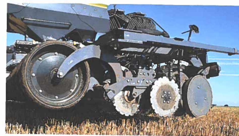
Serrated disc openers are carried in pairs on individual bogey-type coulter carriages with a rubber press wheel up front and smooth steel press rings at the rear.
