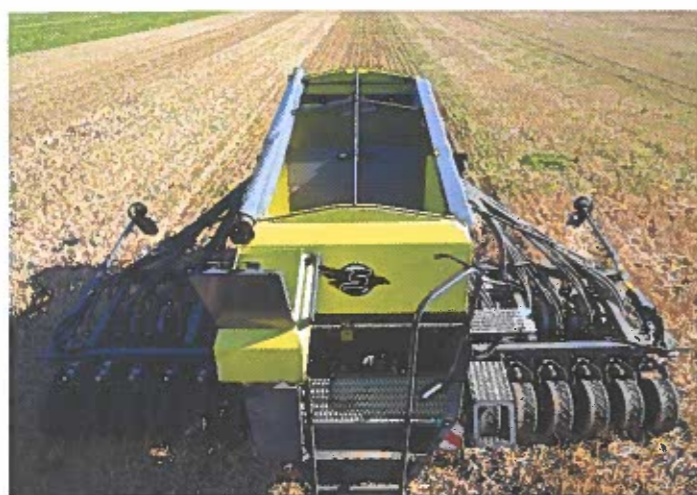
Up front is a small-seed/granule applicator while the main hopper has a 60:40 split and twin metering units for seed and fertiliser.
