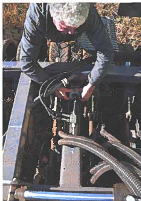
A ram on each wing section sets the fore-aft pitch and weight bias of the coulters to suit soft or hard going.
