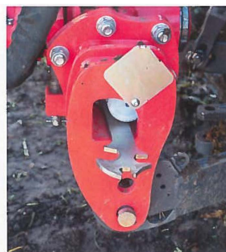
Storage compartment in the headstock frame provides convenient space for plough tools and handbook – no need to carry them in the cab.
