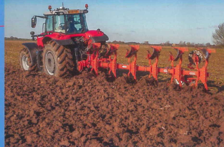
Minimal surface trash and a 95cm point-to-point clearance meant total burial was achievable.
