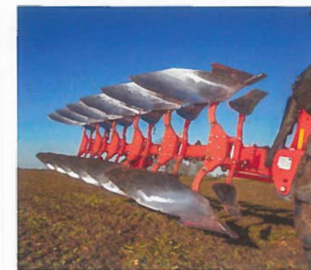
Long-throw MP4WD body is one of two options for the UK. The other option is a slatted board.
