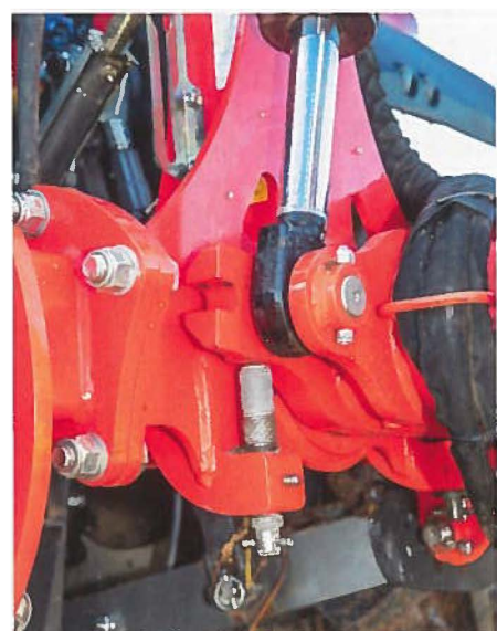
Unico's single turnover ram pushes positively onto adjustable stops.
