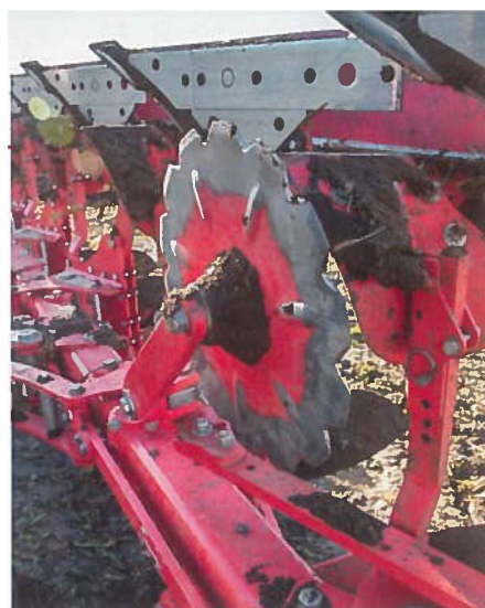
Skimmers are height-adjustable using a pin and clip system – quicker and less fiddly than bolts.
