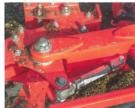
Front furrow adjustment is by turnbuckle; a hydraulic front furrow option is available.
