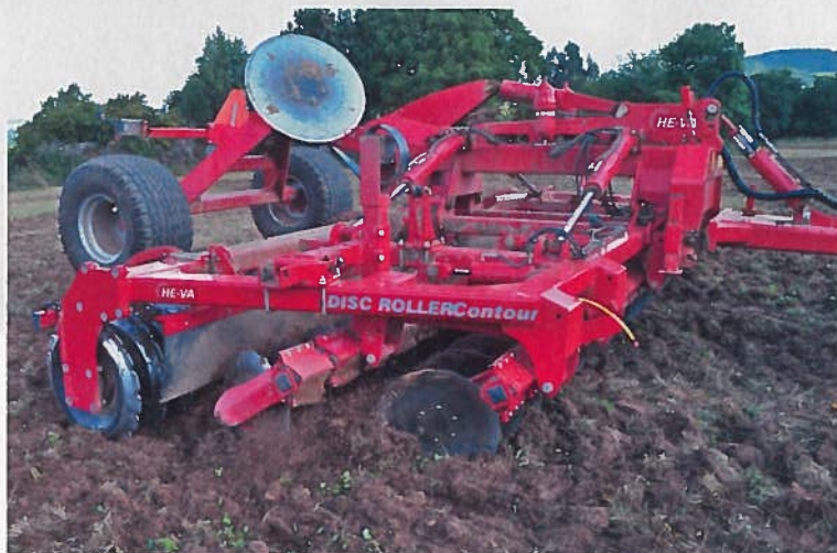
The He-Va Disc Roller Contour being used to disc in an old grass/clover ley – two passes are needed to break up the root systems, but only one is needed for cereal and maize stubble.
