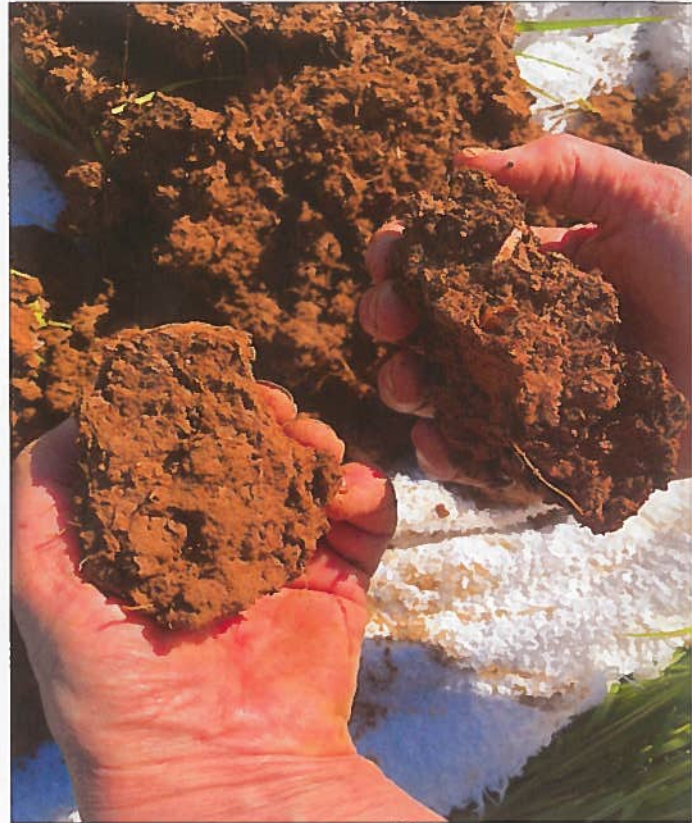
Soil profiles from the trial showing an untreated compacted soil clod in the left hand and subsoil treated soil clod in the right hand.
