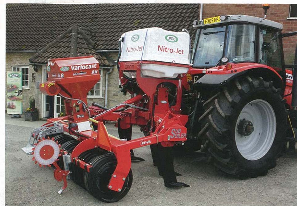
The newest component in Opico's 3m oilseed rape drilling combination is the Synchro roller.
