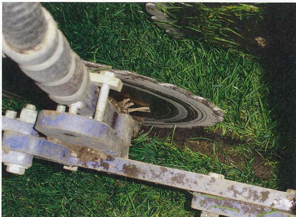
Above: Angled disc on the Moore Unidrill opens a slot for the seed to be dropped into.
