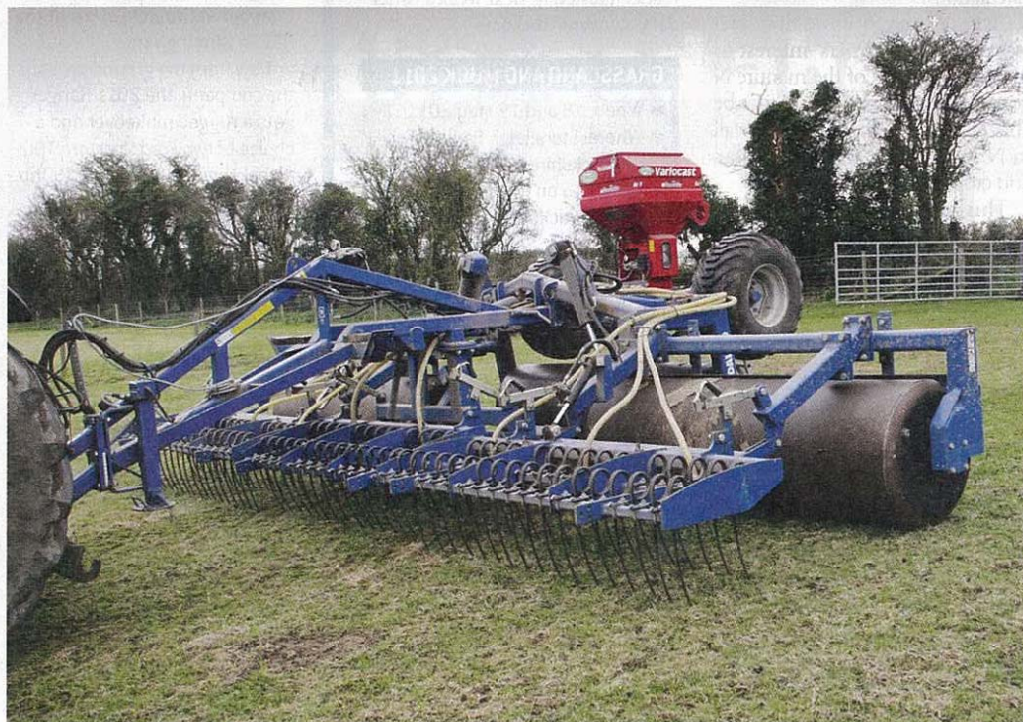
Mike Simpson's Dalbo roller complete with grassland overseeder unit. The tines can be seen raking out matted grass.
