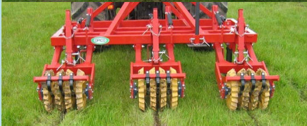
The Swardlifter (above) has been specifically designed for sub soiling grassland
