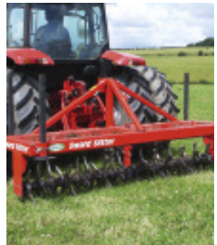
Aerating the ground using a sward slitler combats surface compaction
