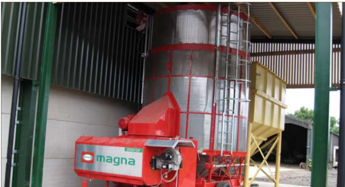
The Opico Magna 200QF offers fully automatic control of its loading, drying, cooling and unloading functions and is housed under a purpose-built lean-to.
