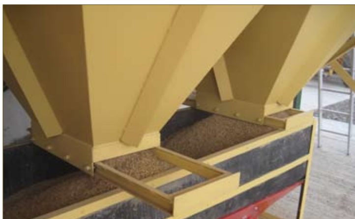
Loading the drier’s holding hopper allows two full batches to be dried over a four-hour period without the need for extra labour. The purpose-made loading hopper’s two outlets sit directly above the drier’s intake auger and help fast filling.
